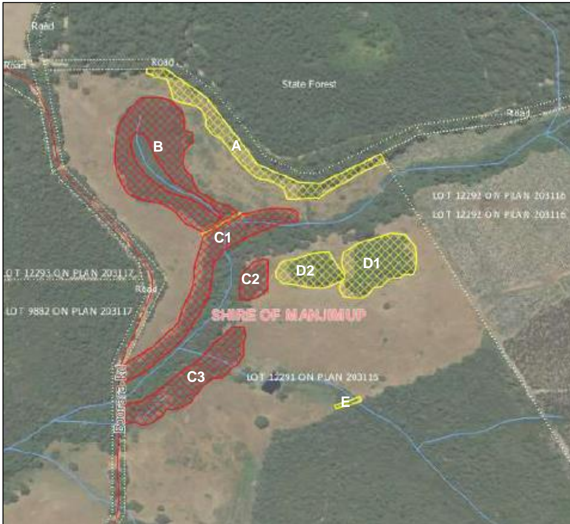
Figure 1 Areas authorised to be cleared under CPS 8830/1 (up to 3.27 ha for broadscale clearing in 'A', 'D' (1-2) and between 'B' and 'C1' shaded yellow, and up to 5.67 ha for 'low impact' / 'incidental' clearing 1 in 'B', 'C' (1-3) and 'E' shaded red) 2
